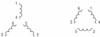
6 Leads, Dual Voltage (1.732:1 Ratio), Wye or Delta Connection
