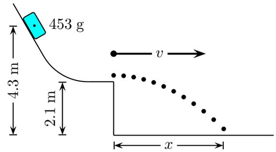
What is the speed of the block when it leaves the track? The acceleration of gravity is  $9.81 \text{ m/s}^2$ .
