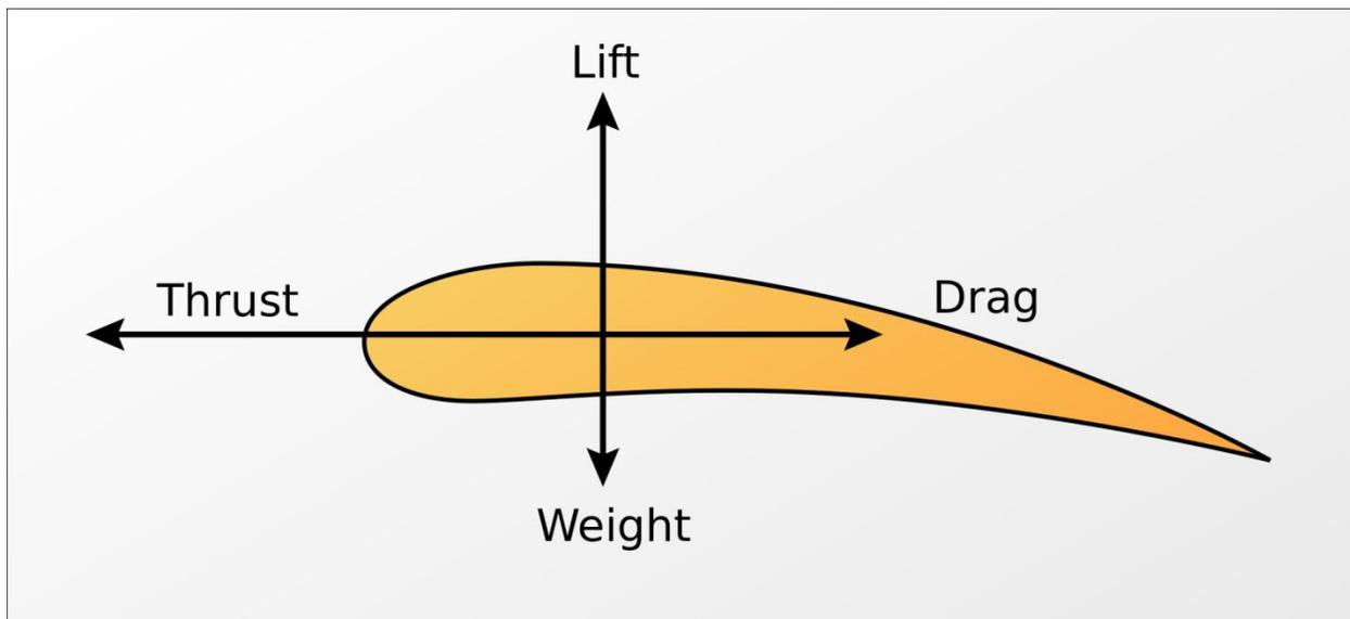
Above is a picture of the four forces acting on an airfoil. An airfoil is also known as a wing.
