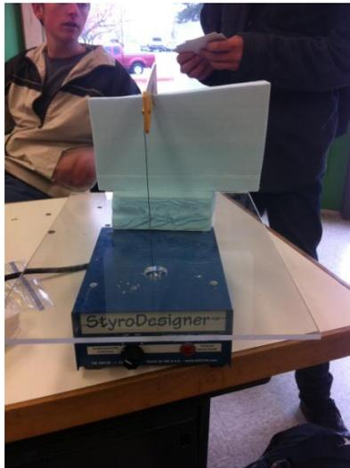
3. Cut a hole for the screw to be able to fit through (Make sure to make the angle of the hole the desired angle of attack)
