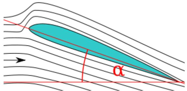
Since we now know how to calculate the lift of the airfoil we now need to find the amount of drag that the airfoil will have. The equation for calculating the drag is the same as the equation for lift, except the coefficient of drag is substituted for the coefficient of lift.
