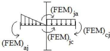
$$\begin{aligned} m_{ja} &= S_{ja} \theta && \text{Sum of the moments must equal} \\ m_{jb} &= S_{jb} \theta && \text{zero, so, } (S_{ja} + S_{jb} + S_{jc} \\ m_{jc} &= S_{jc} \theta && + S_{jd}) \theta = M, \text{ where } M \text{ is the} \\ m_{jd} &= S_{jd} \theta && \text{“external” moment at joint } j \end{aligned}$$
