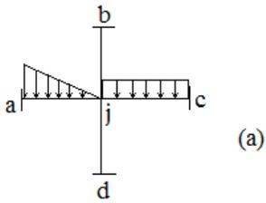
Lock the structure so that there are four fixed-end beams. Find the FEMs, including the total moment  $M$  at the center (ccw). Create an opposite moment shown (cw moment  $M$ ) to “unlock” the beam. Joint  $j$  now rotates through an angle  $\theta$ . Now, picture (e) is equivalent to picture (a) and we can proceed with the moment distribution.
