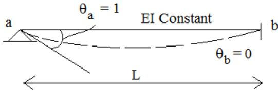
Take the propped-cantilevered beam shown. It has no load. We'd like to know the general relationship between  $\theta_a$  and  $M_{ab}$  (end moment of member ab at "a") or  $M_{ba}$  (end moment of member ab at "b")
