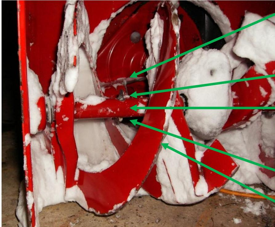
Rotate second stage blades to turn shaft inside auger tube.
