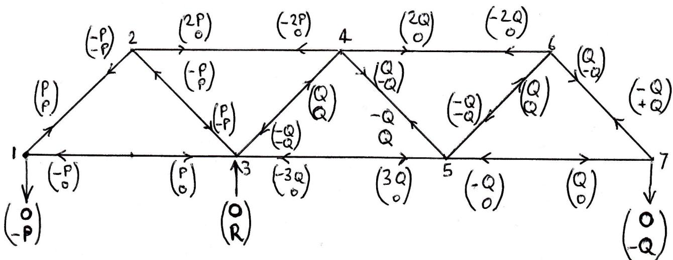
Forces on pins 1-7 are shown as column vectors with x-components on top, y-components underneath.
