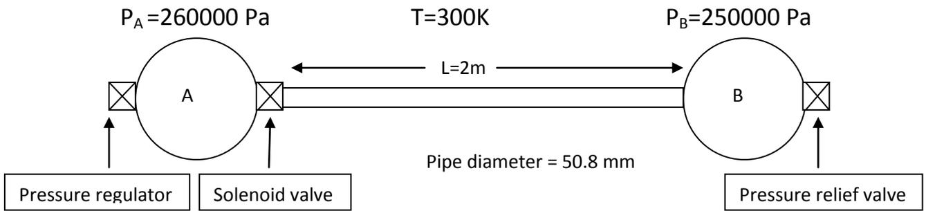
With no flow condition: pressure in Tank A is 260000Pa Tank B and pipe is 250000Pa as shown above
