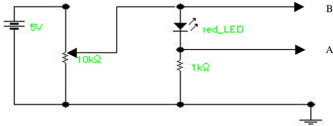
The A input to the 750 interface measures the voltage across the 1000  $\Omega$  resistor in series with the LED. This voltage is directly proportional to the current through the LED, and its value is numerically equal to the current in mA. The B input reads the total voltage across the LED and the 1000  $\Omega$  series resistor. The difference between these two voltages is the voltage across the LED.
