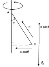
Rod AB has length 0.5 m, and is attached by a frictionless pin at A to a vertical shaft which rotates at 75 rpm.
