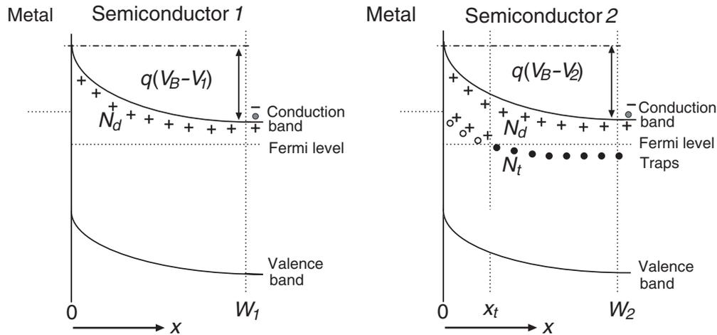
At zero applied voltage ( $V_I = 0$ ) the electrostatic potential difference between metal and semiconductor  $I$  is  $V_B$ . When a voltage is applied the potential difference between metal and semiconductor is  $V_B - V_I$ .
