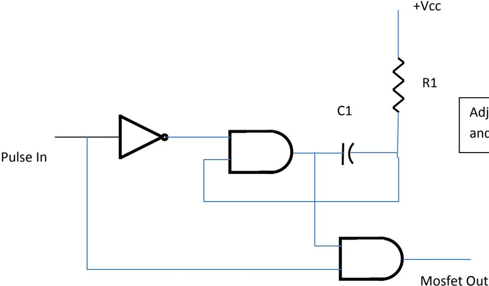
Adjust the values of R2 and C1 for desired delay
