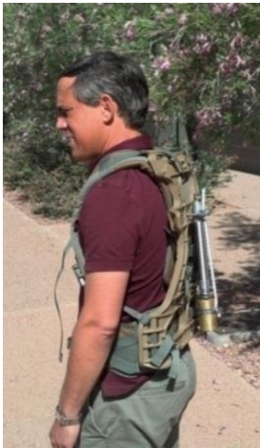
Fig 11: A powered PogoSuit is used to assist the hopping motion. A pneumatic cylinder oscillates the small mass up and down in phase with the user.
