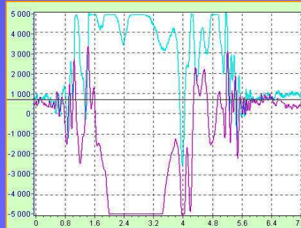
Reflected signal from running human behind two walls.
