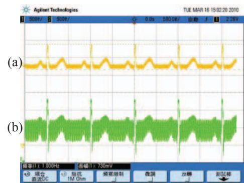
Figure 11. (a) The 60Hz Notch Filter ECG Signal Processing (b) Without 60Hz Notch Filter ECG Signal Processing.
