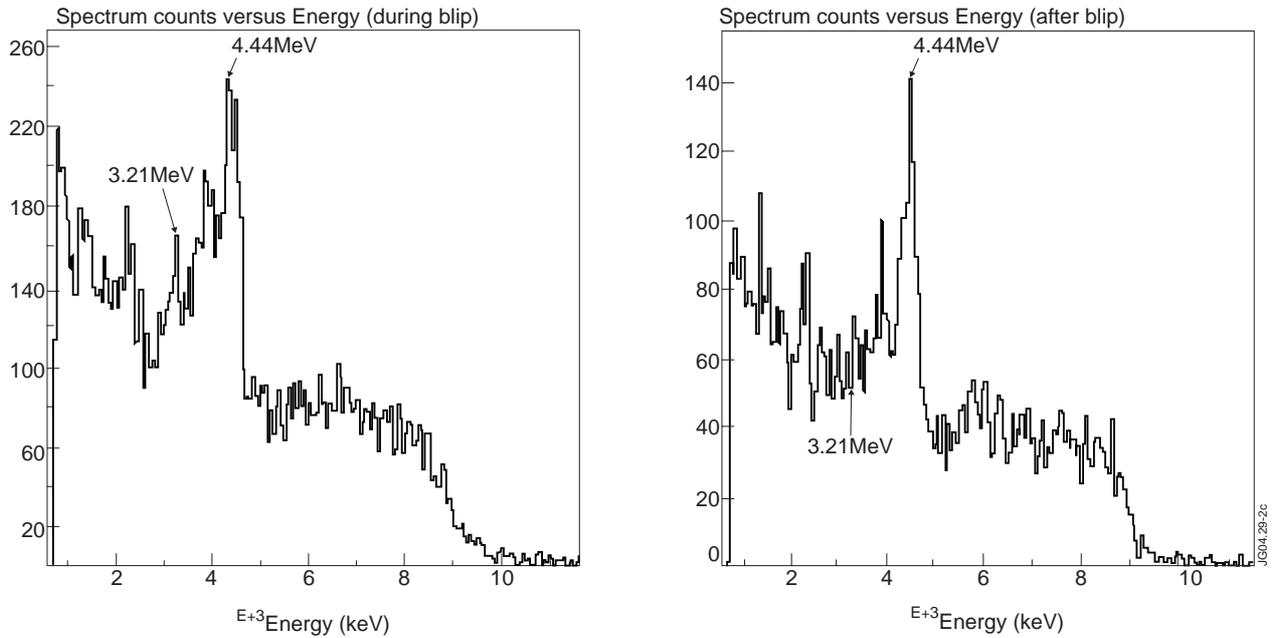
Figure 2: Gamma-ray spectra measured in 2.0 MA/2.25 T Pulse No: 61046 with deuterium 15 MW NBI heating and tritium 300 ms blip  $P_{\text{TNBI}} \approx 1.5 \text{ MW}$ ;  $T_e(0) \approx 6 \text{ keV}$ ,  $n_e(0) \approx 6 \cdot 10^{19} \text{ m}^{-3}$ .
