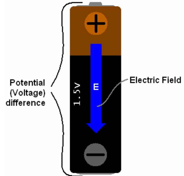
**Figure 3:** in a AA cell, the positive and negative electrodes are separated by a field which creates a potential difference, or voltage, between them. This voltage represents the electric field’s capacity to force charges through an external circuit.
