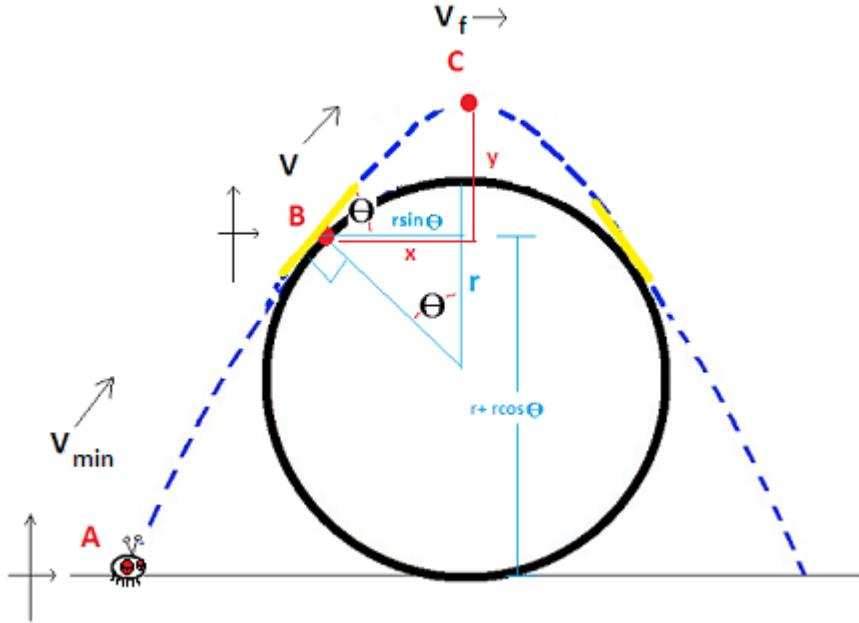
$$\text{A, B: } W_p + f_f S = \Delta K + \Delta U_g + \Delta U_s \rightarrow \Delta U_g = \Delta K$$
