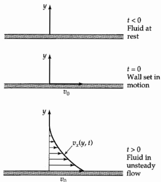
Presumably, the fluid and solid (e.g. cylindrical shell) are at rest at  $t < 0$ , and then are set into motion at  $t = 0$  in the horizontal direction with a velocity  $V$ . Their findings show that, at a time  $t$ , the shear stress exerted by a fluid can be determined by:
