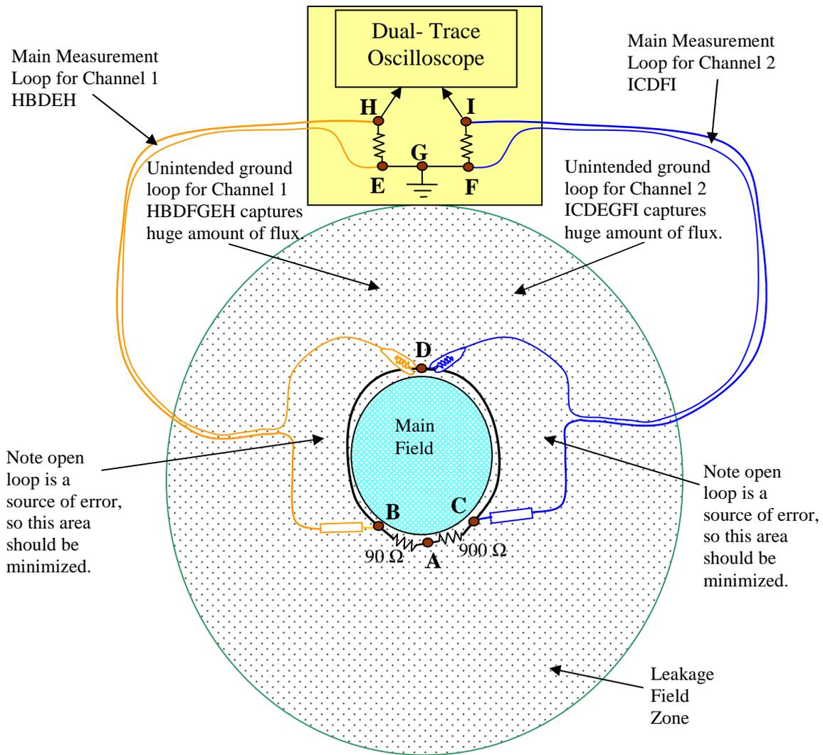
**A Faraday Law Paradox Question:** Notice that the main measurement loop and the unintended ground loop each encircle a different amount of total flux. If either loop were present alone, then the scope would read the emf equal to the time rate of change of enclosed flux. However, with both loops present, what does the scope read, and what is the physical meaning of the value that is given by the scope?
