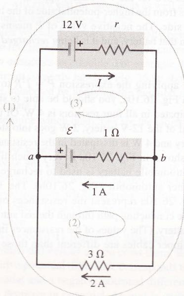
**26.11** In this circuit a power supply charges a run-down battery and lights a bulb. An assumption has been made about the polarity of the emf  $\mathcal{E}$  of the run-down battery; is this assumption correct?
