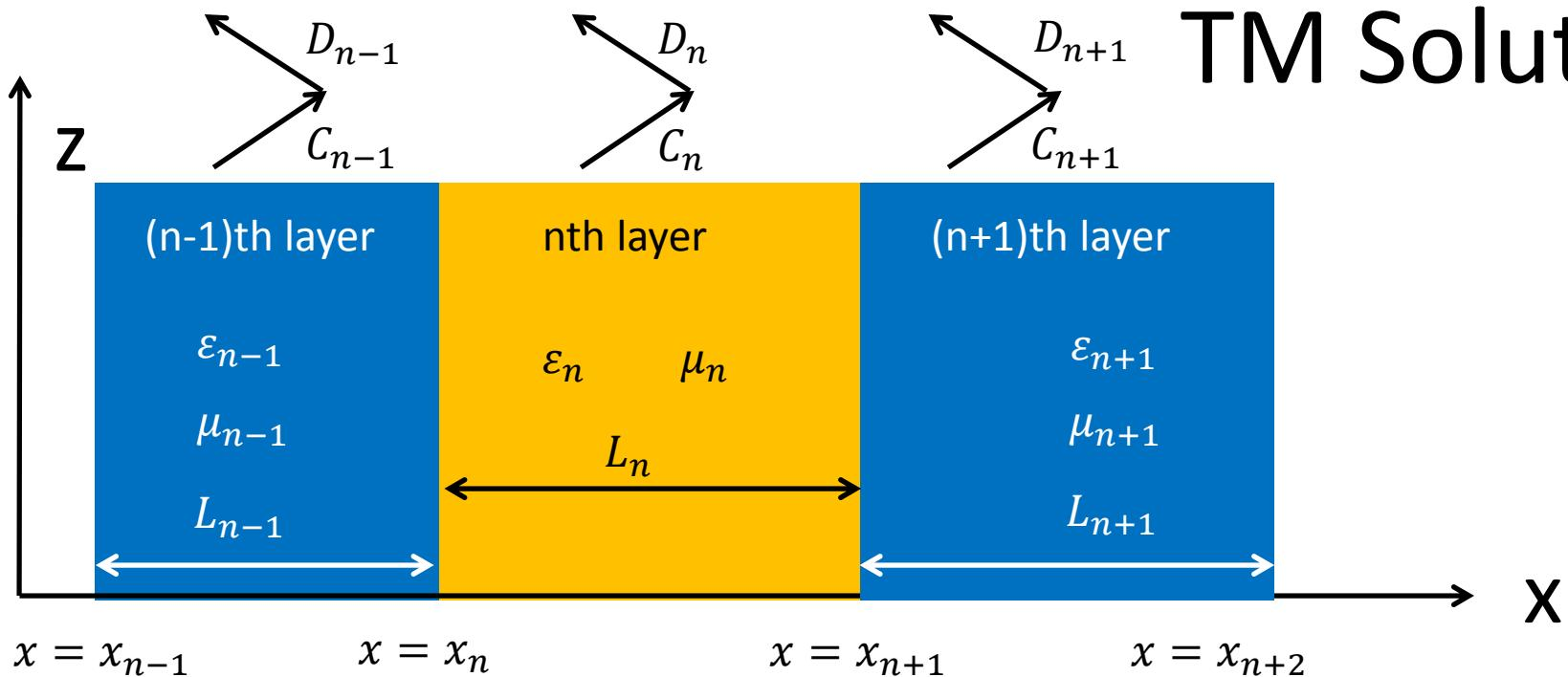
$$\text{nth layer} \quad H_{ny} = e^{j(\omega t - \beta z)} \{C_n e^{-jk_{nx}L_n} + D_n e^{jk_{nx}L_n}\}$$
