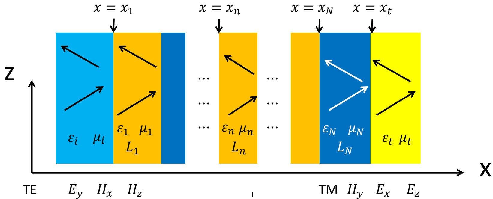
$$r = \frac{(T_{TE}^{-1})_{21}}{(T_{TE}^{-1})_{11}}$$
