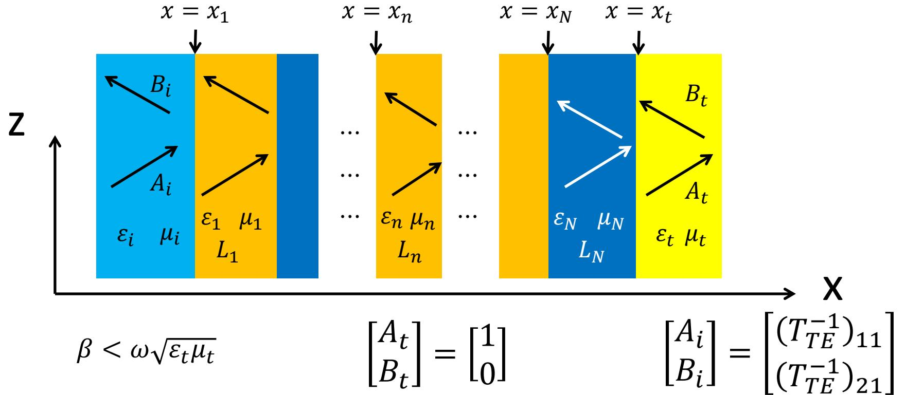
$$T = \frac{S_{tx}}{S_{ix}} = \frac{\frac{k_{tx}}{2\omega\mu_t} |A_t|^2}{\frac{k_{ix}}{2\omega\mu_i} |A_i|^2} = \frac{\mu_i k_{tx}}{\mu_t k_{ix}} \frac{1}{|(T_{TE}^{-1})_{11}|^2}$$
