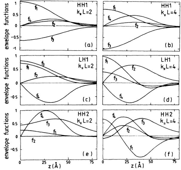
FIG. 3. Envelope-function components of the three highest subbands in the  $\langle 10 \rangle$  direction in a 100-Å GaAs-Ga<sub>0.79</sub>Al<sub>0.21</sub>As quantum well without stress. The wave functions have been calculated for  $k_{\parallel}L=2$  and  $k_{\parallel}L=4$ .
