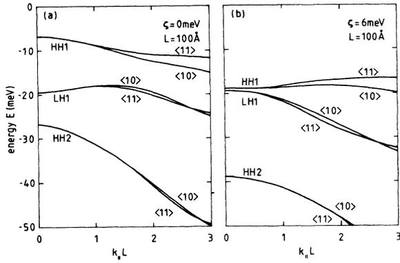
FIG. 2. Dispersion of the three highest valence subbands in a GaAs-Ga<sub>0.79</sub>Al<sub>0.21</sub>As quantum well of width  $L=100$  Å, (a) with no stress ( $\zeta=0$ ) and (b) with an applied stress  $X=2.3$  kbar ( $\zeta=6$  meV). In (b) the zero of the energy has been taken to coincide with the top of the bulk GaAs valence band under the same stress.
