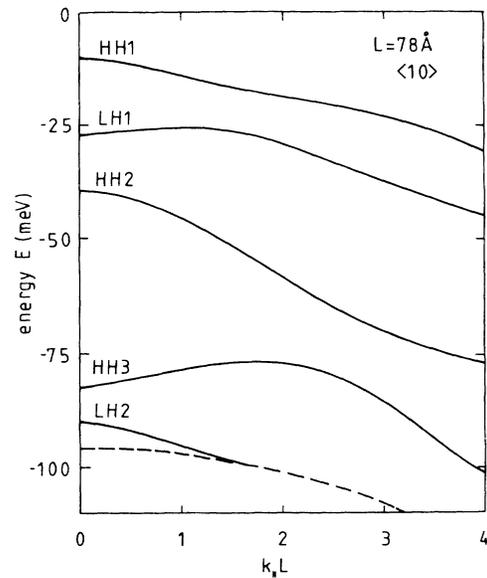
FIG. 5. Confined hole levels in the  $\langle 10 \rangle$  direction for a 78-Å GaAs-Ga<sub>0.79</sub>Al<sub>0.21</sub>As quantum well. The dashed line marks the onset of the continuum; the well barrier depth is  $-V_0 = -95.65$  meV.
