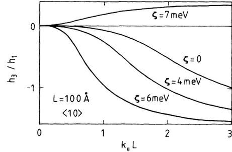
FIG. 4. Ratio  $h_3/h_1$  for the HH1 subband of a 100-Å GaAs-Ga<sub>0.79</sub>Al<sub>0.21</sub>As quantum well in the  $\langle 10 \rangle$  direction, for the values  $\zeta=0,4,6,7$  meV of the stress parameter.
