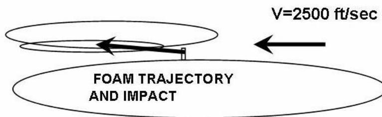
The incident occurred at an altitude of 65600 ft where the atmospheric density is .000171 slugs/cu ft. The velocity of the shuttle was 2500 fps. The foam block had a cross sectional area of 1 sq ft and a weight of 2 lbs. Assume a drag coefficient  $CD=1.25$ .
