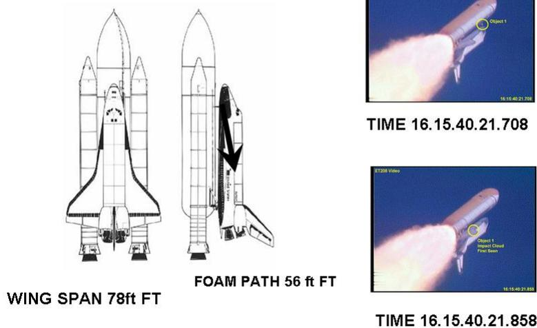
The space shuttle Columbia was damaged on liftoff when a piece of insulating foam from the bipod ramp that holds the shuttle to the external tank came loose, accelerated in the air flow and hit the leading edge of the wing. The wing span of the shuttle is 78 ft. Use 56 ft. as your estimate of the flight path length of the foam in the air stream (see figure).
