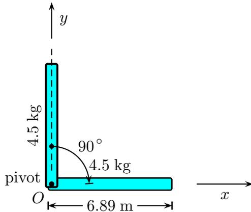
At the instant the rod is horizontal, find its angular speed. The acceleration of gravity is  $9.8 \text{ m/s}^2$ . Answer in units of  $\text{rad/s}$ .
