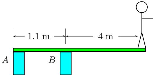
Find the force on the support *A* when a 70 kg diver stands at the end of the diving board. Answer in units of kN.
