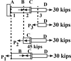
Applying FBD analysis to each component to find internal forces.
