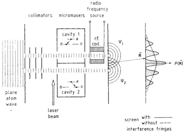
FIG. 6 Asymmetric set-up in which cavity 1 induces the transition  $a \rightarrow b$  and cavity 2 induces  $a \rightarrow c$ . Which-path information is erased by the radio frequency in the coil where  $b \rightarrow c$  happens.
