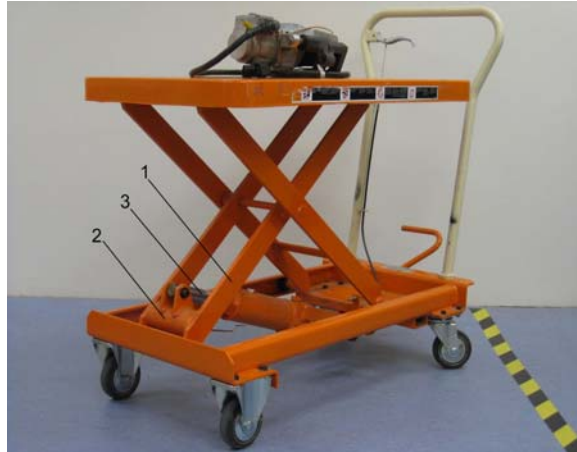
(a) A scissors lift table with 250 kg SWL (Safe Working Load) is loaded with a prototype electromechanical brake.
