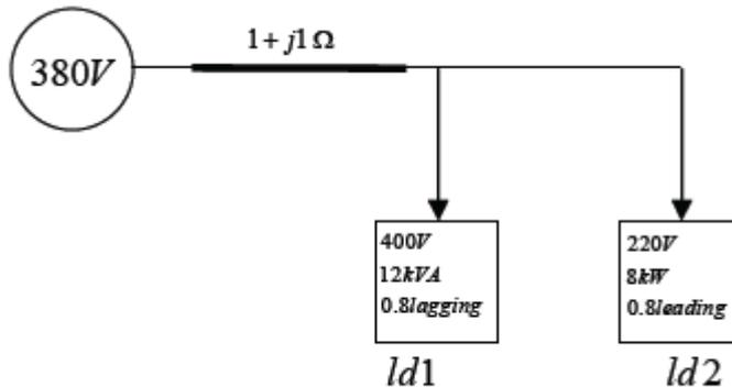
Calculate the current through the transmission line (magnitude and phase).
