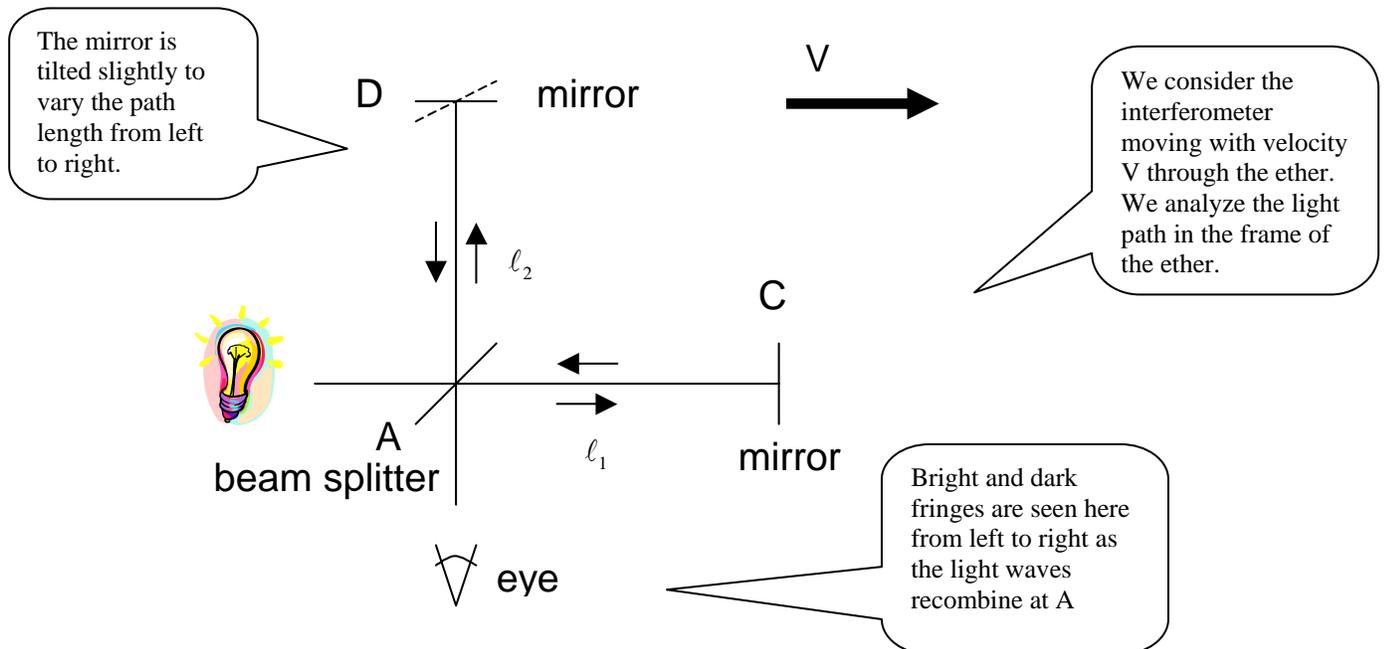
Calculate the time it takes to travel the horizontal path from A ↔ C:
