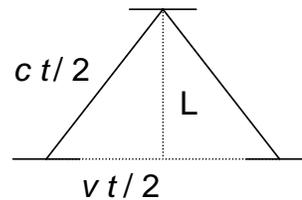
So the time it takes the light pulse to make a roundtrip in the clock when it is moving by us appears longer than when it is at rest. We say that time is **dilated**. It also doesn't matter which frame is the Earth and which is the clock. Any object that moves by with a significant velocity appears to have a clock running slow. We summarize this effect in the following relation:
