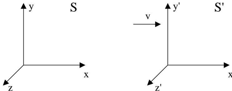
Now suppose that there is a single flash at the origin of  $S$  and  $S'$  at time  $t = t' = 0$ , when the two inertial frames happen to coincide. The outgoing light wave will be spherical in shape moving outward with a velocity  $c$  in *both*  $S$  and  $S'$  by Einstein's Second Postulate.
