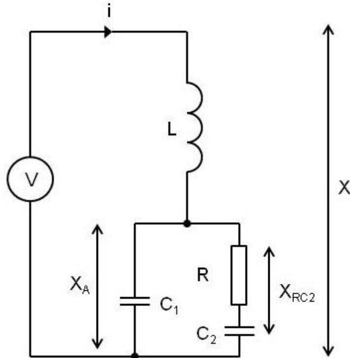
Let:  $X_{RC2}$  be the impedance of the series combination R plus  $C_2$ .
