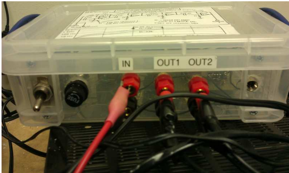
Figure 4a. Front of completed circuit in enclosure.
