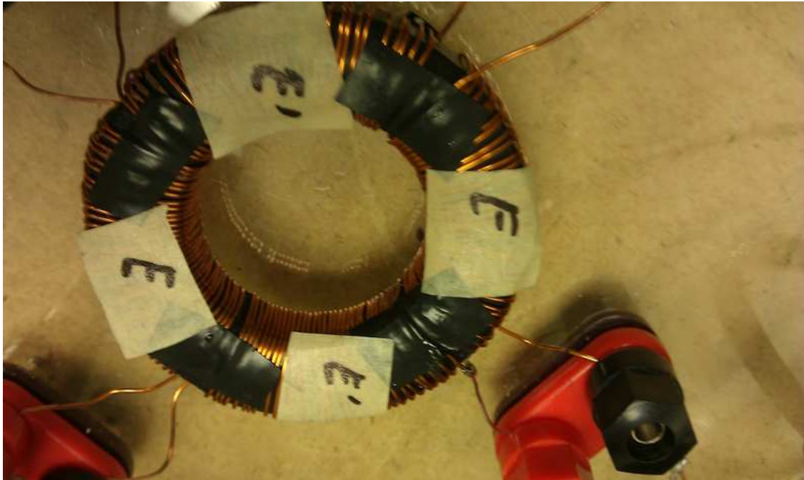
Figure 7 Picture of toroid coil with single layer winding and labeling.
