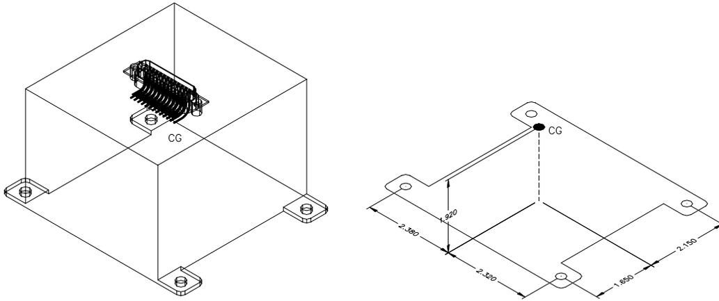
It is assumed the unit acts as a rigid body and that, due to the relative centricity of the center of gravity, that the load applies equally to each of the four screws. Therefore, the tensile and shearing forces on each screw will be represented by:
