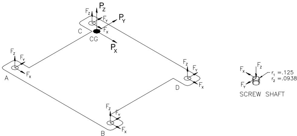
The load applied is an ultimate load case at 20g acceleration in the lateral, longitudinal and vertical directions. The weight of the unit is assumed to be 2.80 lbs maximum, resulting in a force of 56lb<sub>f</sub> for each direction tested.
