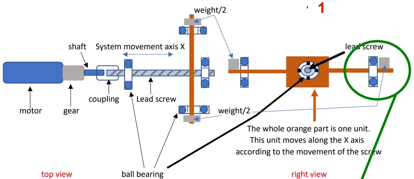
The orange part don't rotate around the screw .
