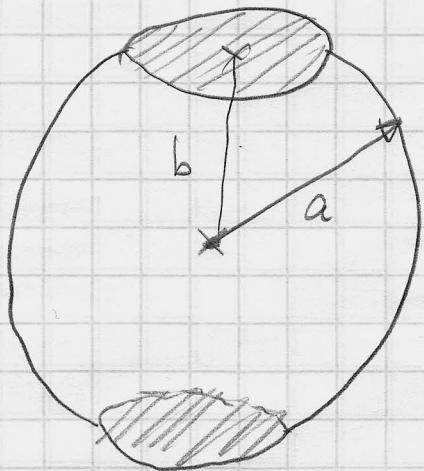
A sphere of radius  $a$  is truncated with a flat plane chord at radius  $b$  ( $b < a$ ), at both ends symmetrically. What is the resistance from end to end?
