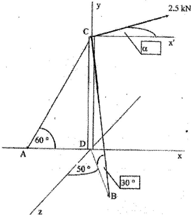
Two wires  $AC$  and  $BC$  are attached to the top of pole  $CD$ . The force exerted by the pole at  $C$  is vertical and the  $2.5 \text{ kN}$  force applied at  $C$  is horizontal and makes an angle  $\alpha$  with the direction of the  $x$ -axis.
