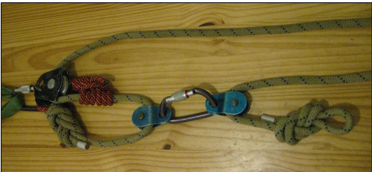
Figure 4: A picture of the DLC attached to a second counterbalance system, minus a tether between the patient and the rescuer.
