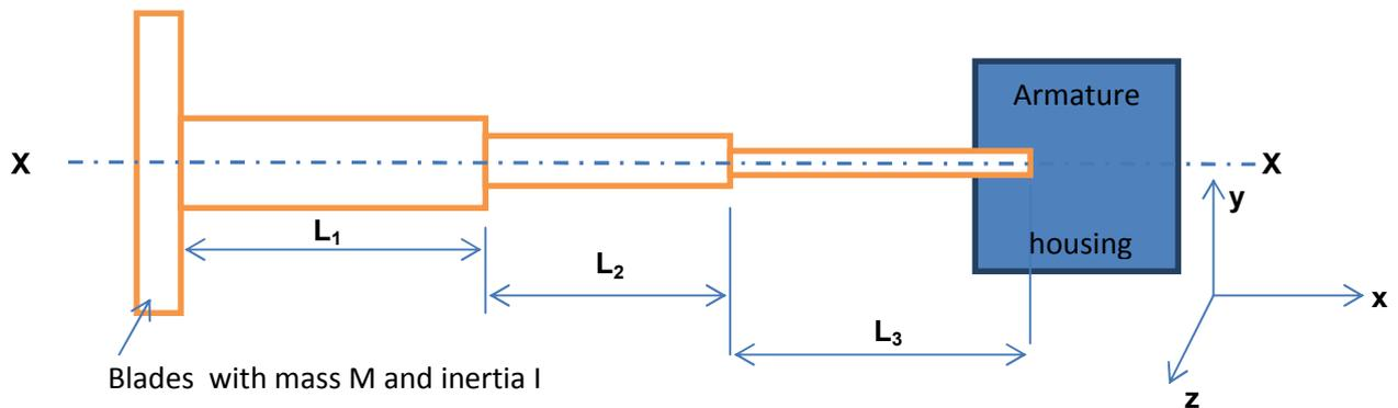
Wind hits the turbine blades with a pressure  $P$  Pa in a direction which may be averaged out at 90 degrees to the y-axis, creating a torque  $T_a$ , which acts clockwise in the x-direction as we look at the diagram from the left hand side.
