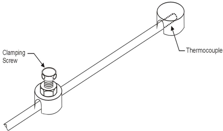
monitoring range, quick response, high accuracy, small size, and rugged construction. Their size and ruggedness make them excellent for measurements in remote or otherwise inaccessible locations.
