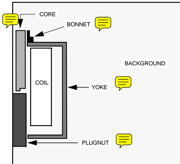
The 2D diagram actually represents a 3D structure that has been revolved around an axis of symmetry, as shown in the
