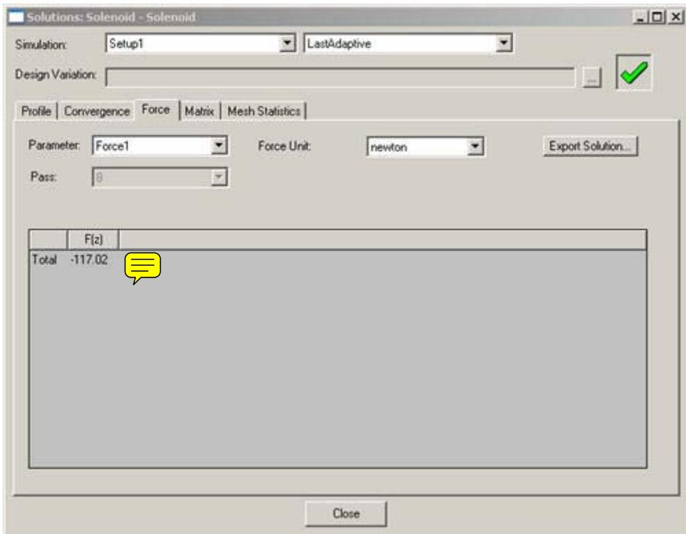
The net force on the core is approximately 117 newtons, acting in the negative Z direction (pulling the core down into the solenoid). There is no component of force in the R direction because of the axial symmetry. Click Close to dismiss the window.
