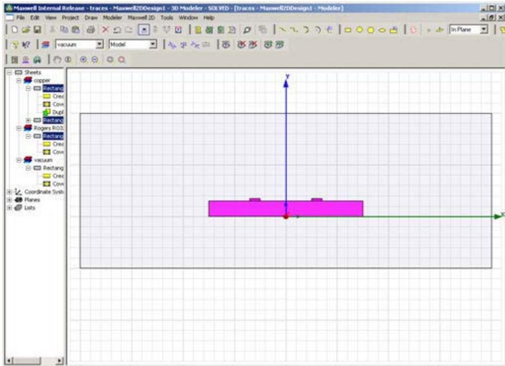
This model is actually a three-dimensional (3D) object. Maxwell 2D analyzes the 2D geometry as a cross-section of the model, then generates a solution for that cross-section.
