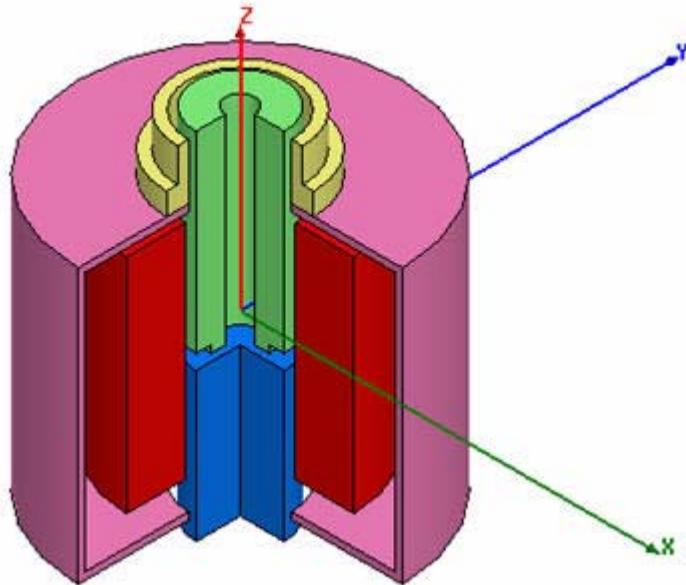
Since the cross-section of the solenoid is constant, it can be modeled as an axi-symmetric model in Maxwell 2D. Of course, material properties, excitations and boundary conditions must also be appropriately modeled by an axi-symmetric design.
