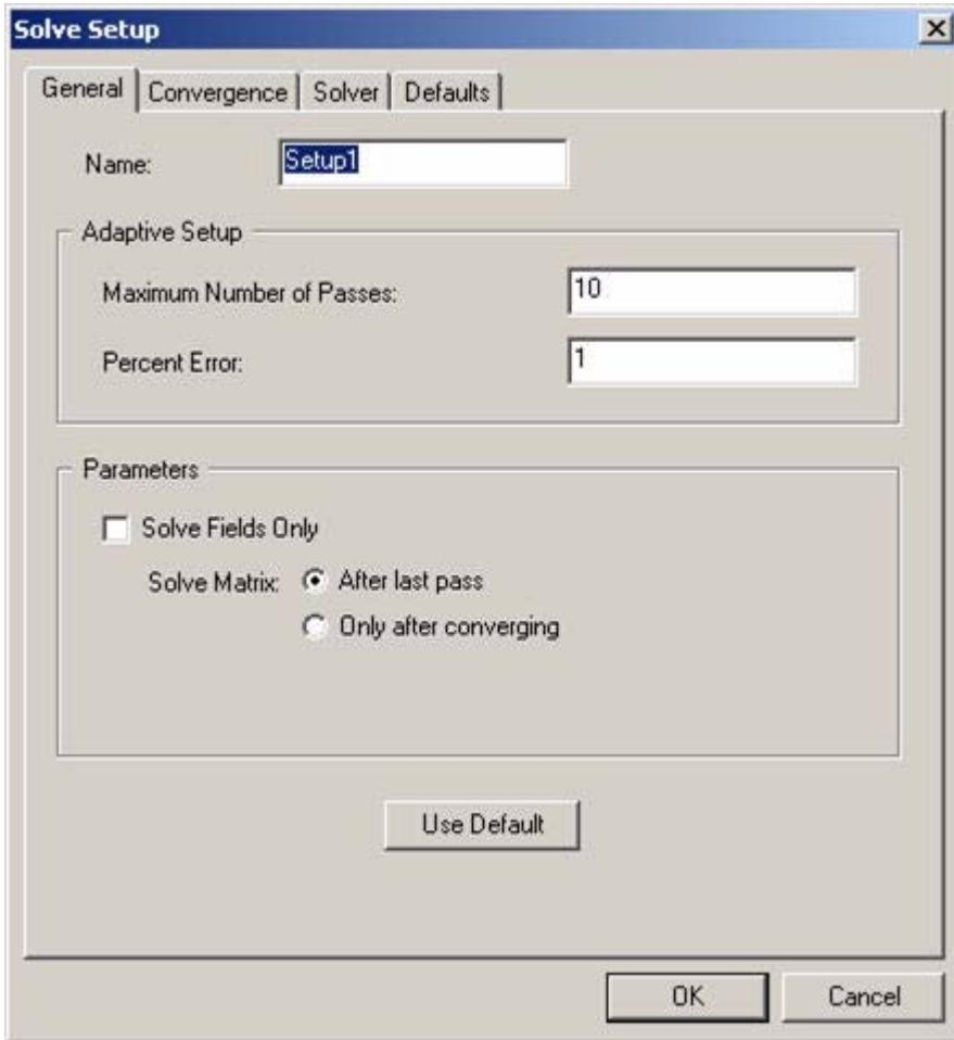
When the system generates a solution, it explicitly calculates the field values at each node in the finite element mesh and interpolates the values at all other points in the problem region.
