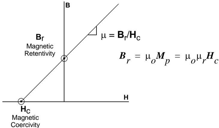
The values of the other two properties, magnetic retentivity,  $B_r$ , and magnetization,  $M_p$ , are computed using the relationships shown above. You may use the "Calculate Properties for" pull down to calculate one set of properties from the other.
