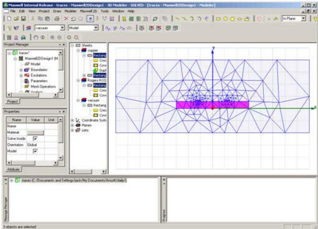
Dividing a structure into many smaller regions (finite elements) allows the system to compute the field solution separately in each element. The smaller the elements, the more accurate the final solution.
