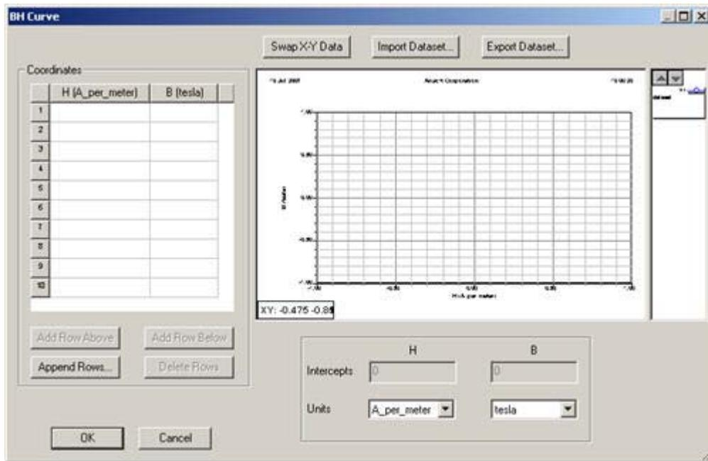
On the left is a blank BH-table where the B and H values of individual points in the B-H curve are displayed as they are
