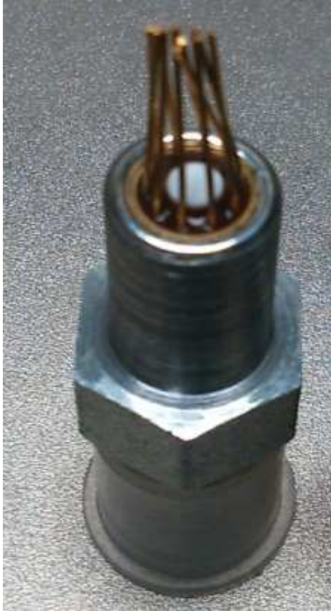
Pictures of the sample, Steel case and TO Header made of KOVAR
