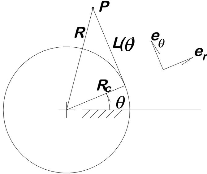
Particle on a Cord Winding Onto a Cylinder
