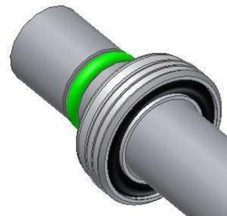
Insert Sample Tube into the Lower Piston Rod/Capture Tube Assembly.
