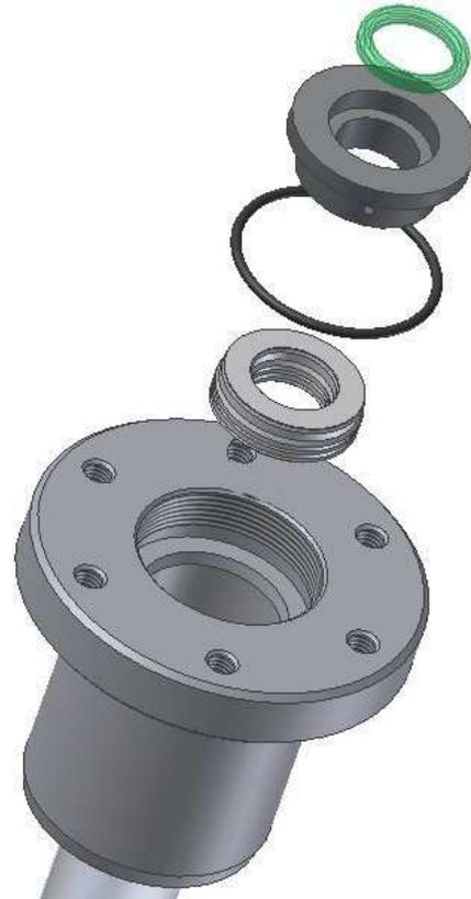
**8.5.10 Reassembly of Piston/Sample Tube Actuator/Lower Piston Rod Assembly**
