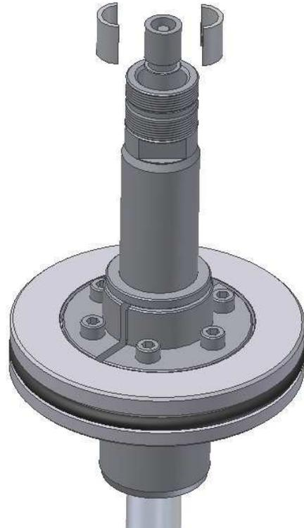
Unscrew the 6 off M5 x 20mm cap head screws (33), remove the Catchplate (17) and Actuator (16) from the Piston (15).
