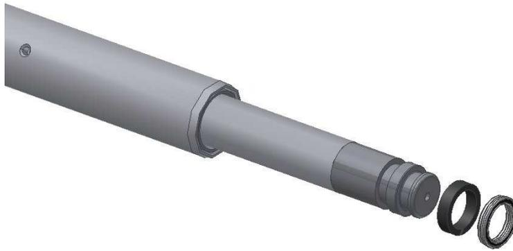
Push the top end of the Sample Tube (94) down until the Sample Tube Balseal (79) and Slydring (80) are exposed at the opposite end of the Sample Tube.
